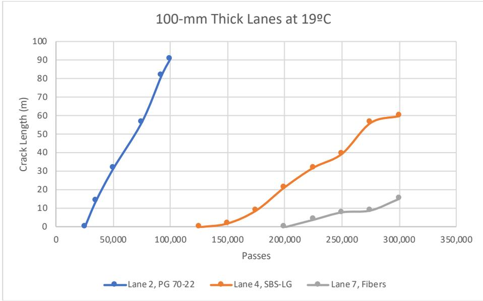
Figure 3. Cracking Length of 100-mm Lift Thickness at 19°C. [5]
