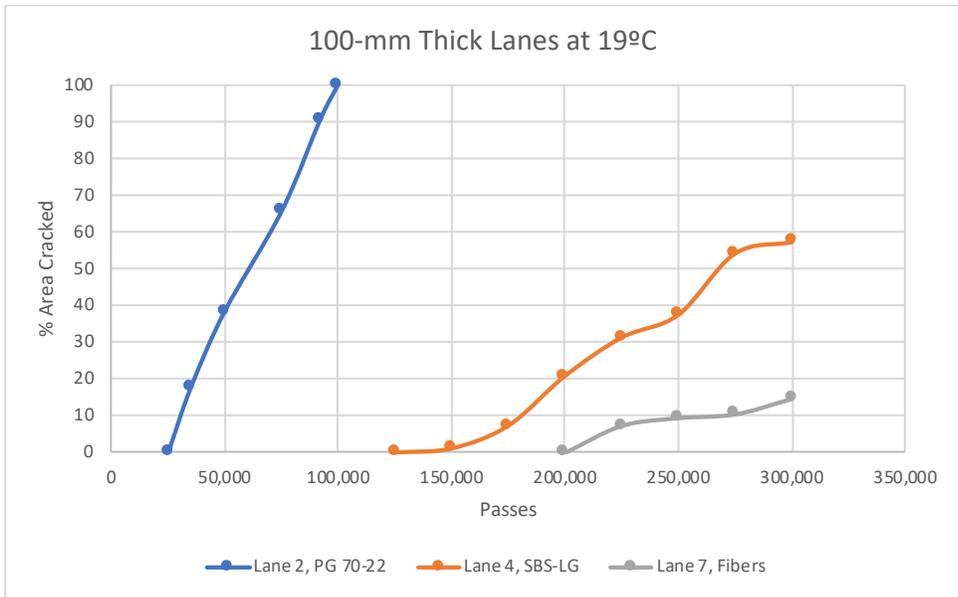
Figure 4. Percent Area Cracked of 100-mm Lift Thickness at 19°C [5]
