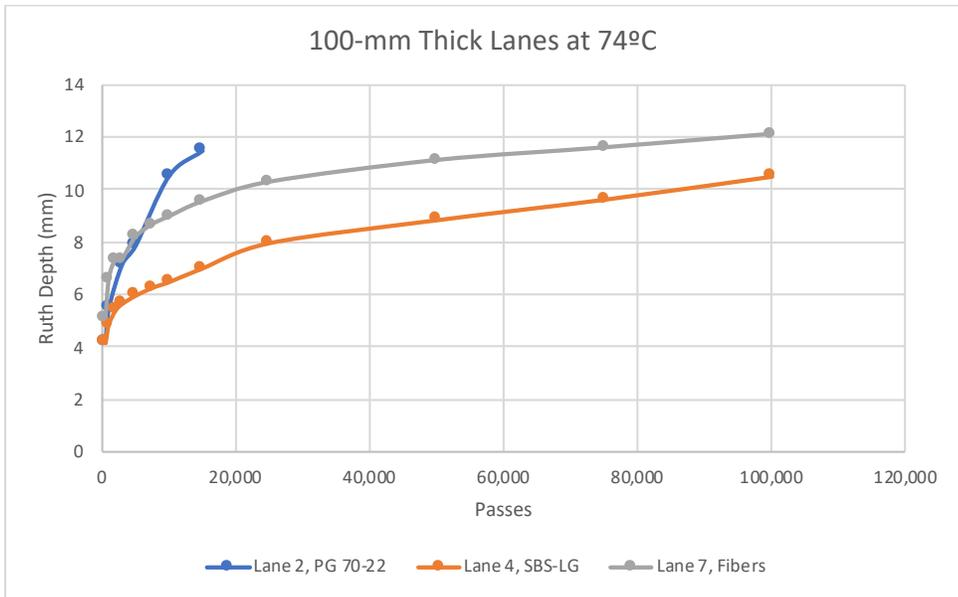
Figure 2. Rutting Data of 100-mm Lift Thickness at 74°C [5]
