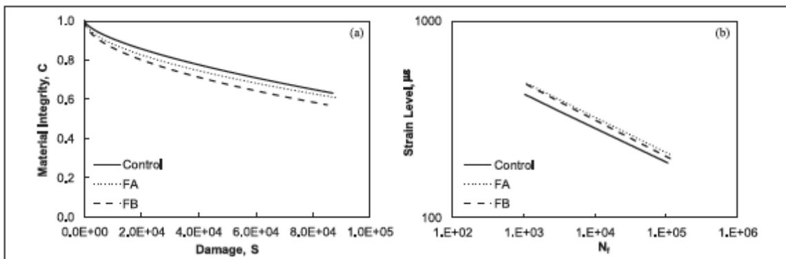
Figure 7. Uniaxial Fatigue Evaluation [7]
