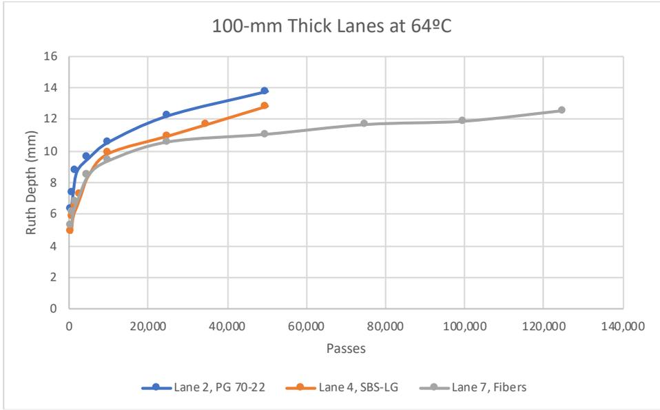
Figure 1. Rutting Data of 100-mm Lift Thickness at 64°C [5]
