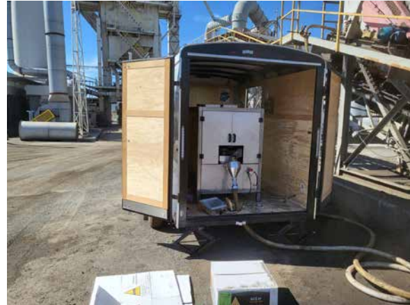
The DFNDR is transported in a trailer so it can set up anywhere at the plant
