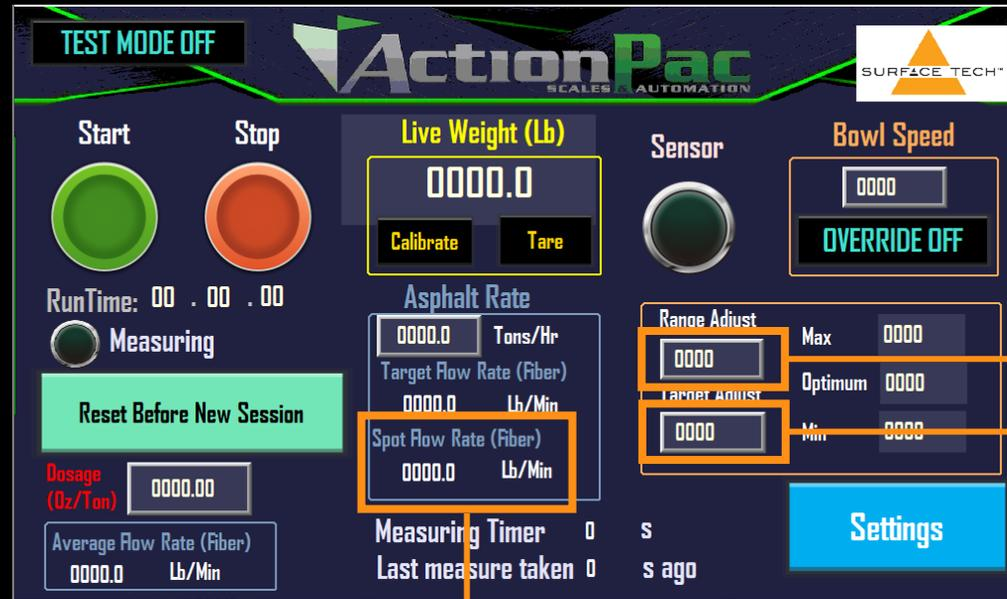
It is recommended to start the Range Adjust at **6** and Target Adjust at **0**. If you feel the Optimum Bowl Speed is undervalued or overvalued, you may change Target Adjust + or - numbers respectively
