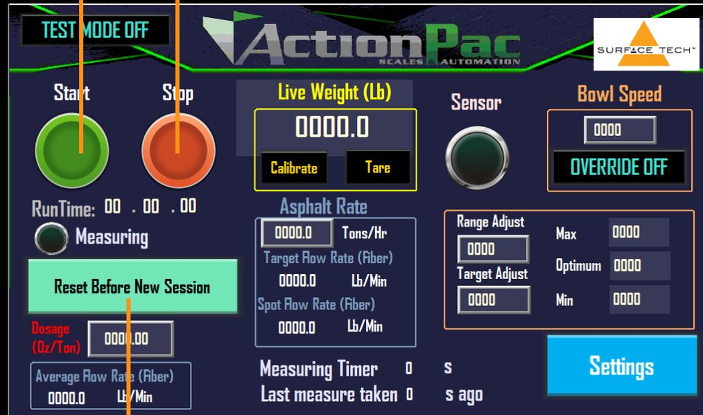
Before initial start-up, and between any changes in plant rate, press 'Reset Before New Session' to ensure continuous accuracy.
