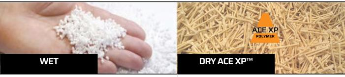
Wet polymers are usually synthetic materials like styrenebutadiene-styrene (SBS), crumb rubber (CR), ethylene-vinyl acetate (EVA), or polyethylene (PE). The addition of polymers to the asphalt binder helps to create a more robust, durable, and flexible pavement material.
