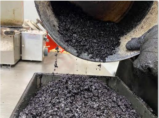
Step 8 – After mixing, split mix into three pans for conditioning. Each pan should contain enough material to compact one IDEAL-CT or HWT specimen.
