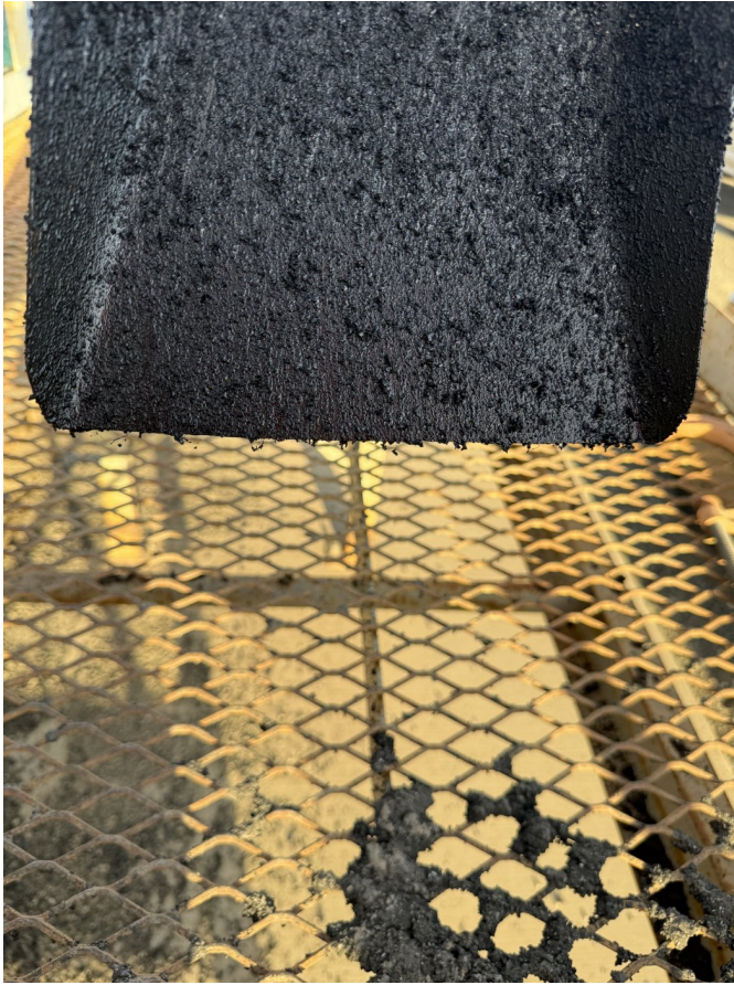
Fiber-reinforced mix sample — uniform dispersion through the ½" HMA.
