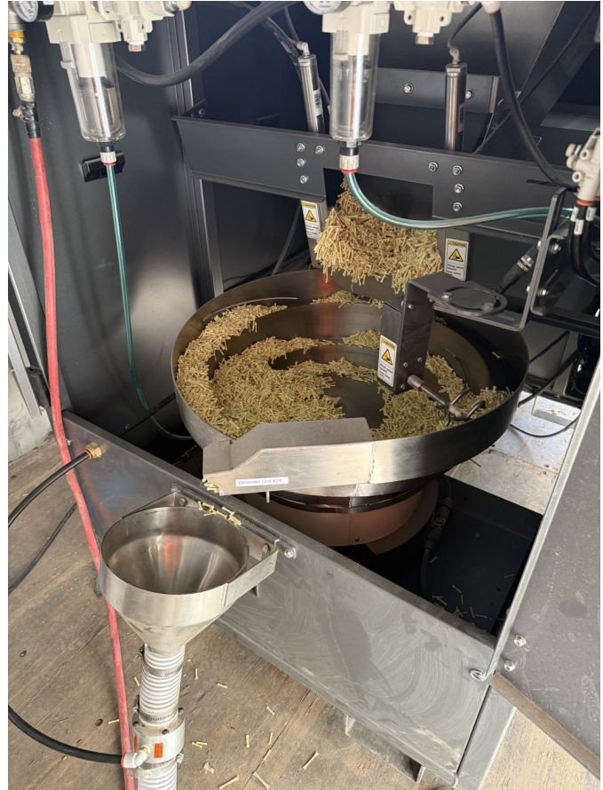
Fiber metering in progress – consistent single-dose delivery batch after batch.
