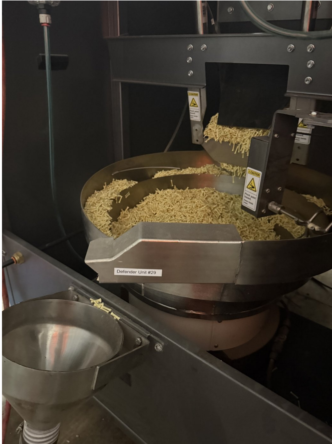
ACE XP fibers feeding through the Defender's metering bowl into production.
