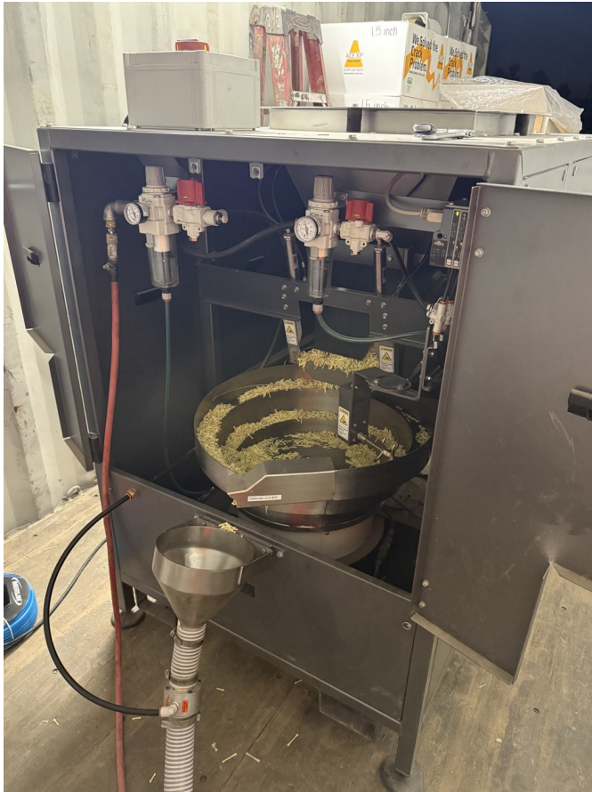
The Defender dosing unit charged with ACE XP aramid fibers at Teichert Woodland.
