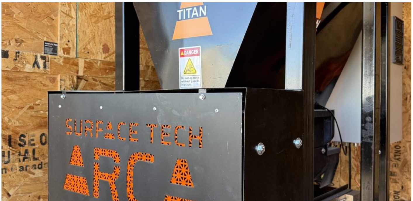
Surface Tech's TITAN dosing unit metering ACE XP fibers into production at Vulcan Materials' Santa Ana plant
