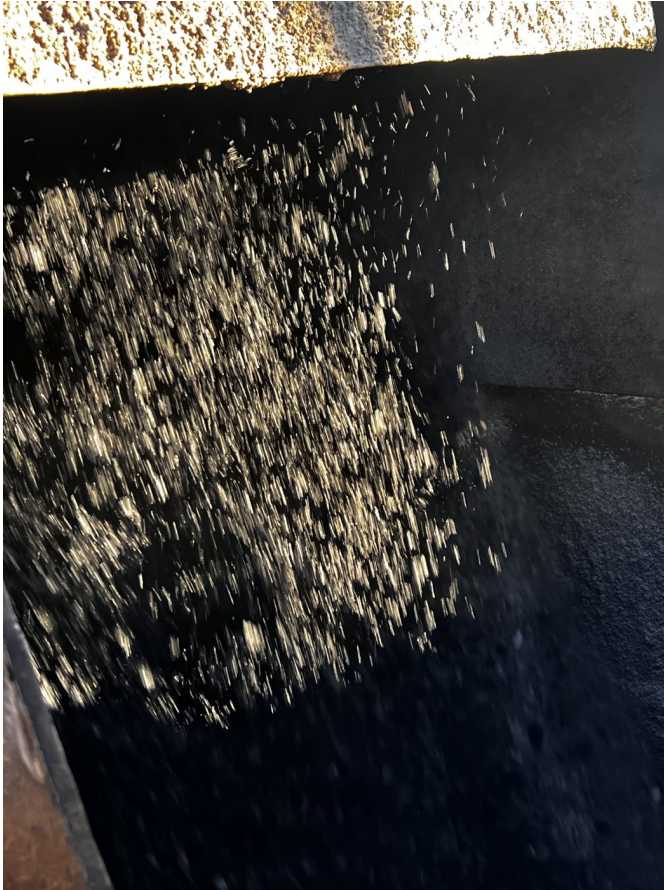
Single-dose fiber addition metering into the 64-22, 25% RAP B mix.
