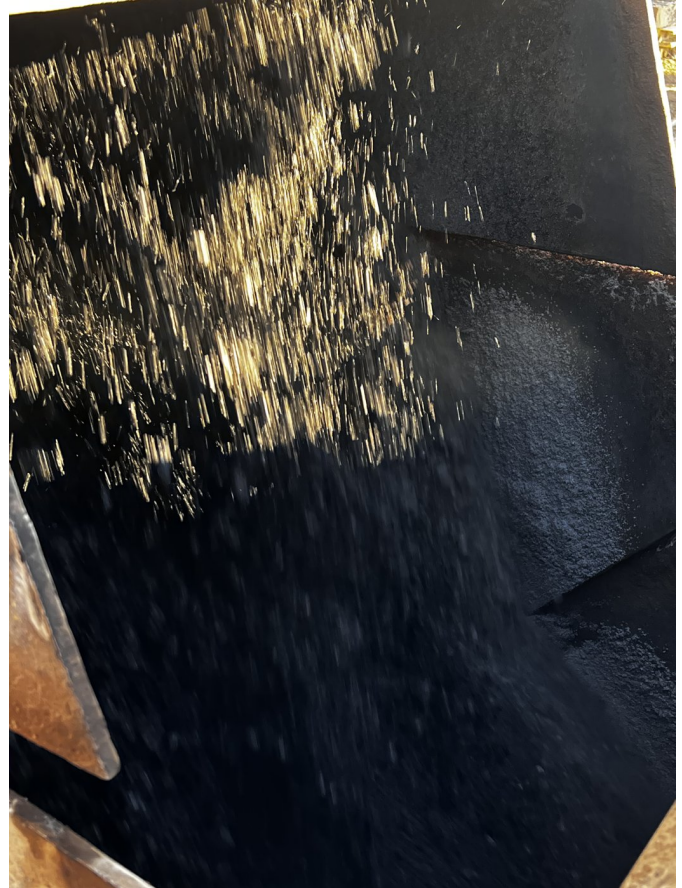
ACE XP aramid fibers dispersing into the mix stream during plant production.
