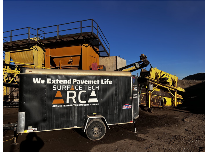
The ARCA dosing unit integrated with the West Plant's production line.
