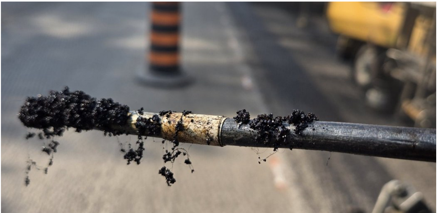
Fiber-laden mix at the paving train — County Road 27 placement, Simcoe County, ON
