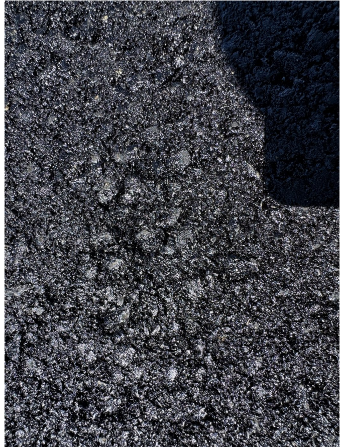
Mix texture close-up: ½" PG 64-16 with 25% RAP and ACE XP 38mm fiber.
